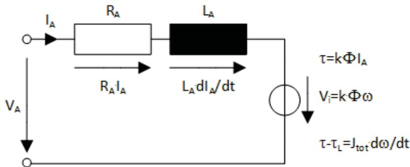
$$T_A = \frac{L_A}{R_A} \rightarrow \frac{V_A - V_i}{R_A} = I_A + T_A \cdot \frac{dI_A}{dt}$$
