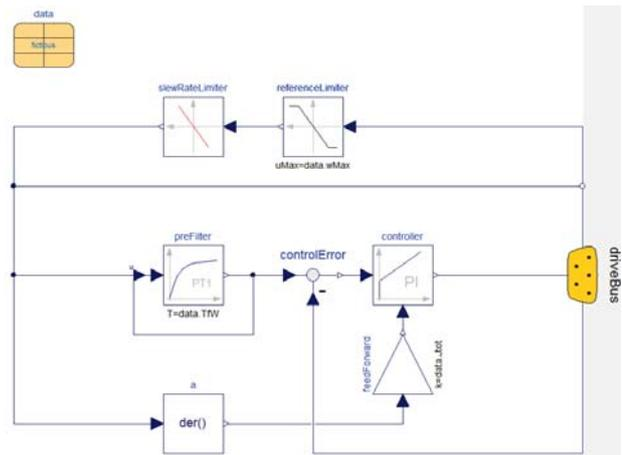
$$\frac{\omega_{Act}}{\omega_{Ref}} = G_F \cdot \frac{G_C G_D}{1 + G_C G_D} = \frac{1}{1 + s4T_{sub} + s^2 8T_{sub}^2 + s^3 8T_{sub}^3} \approx \frac{1}{1 + s4T_{sub}}$$
