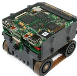
Figure 1: Intelligent Miniature Robot BeBot
