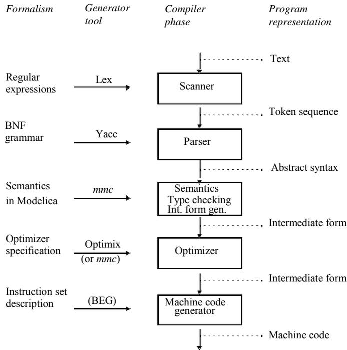
**Figure 1-1.** Generation of implementations of compiler phases from different formalisms. MetaModelica is used to specify the semantics module, which is generated using the mmc tool (MetaModelica Compiler).
