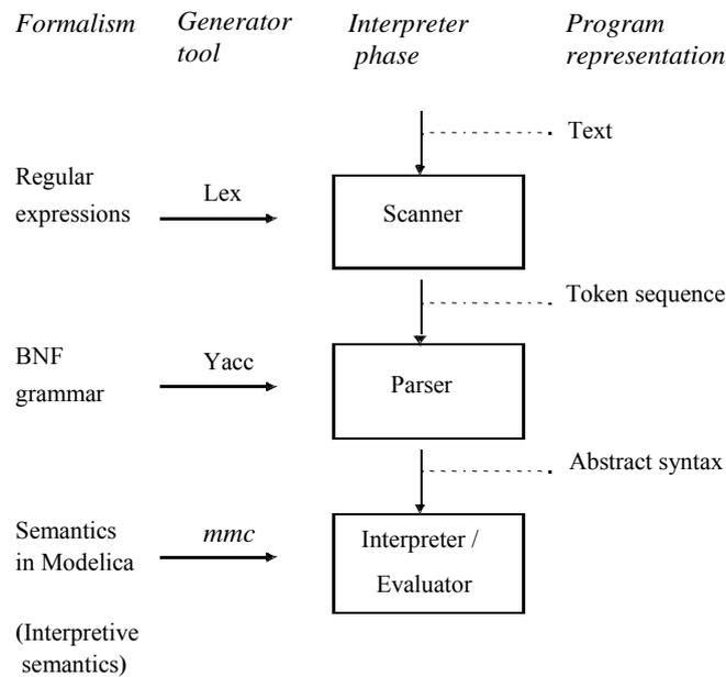
**Figure 1-2.** Generation of a typical interpreter. The program text is converted into an abstract syntax representation, which is then evaluated by an interpreter generated by the MetaModelica Compiler (*mmc*) system. Alternatively, some other intermediate representation such as postfix code can be produced, which is subsequently interpreted.
