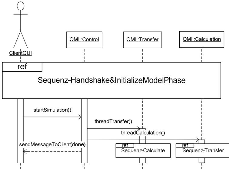
**Figure 6-5 UML-Seq Simulation start**
