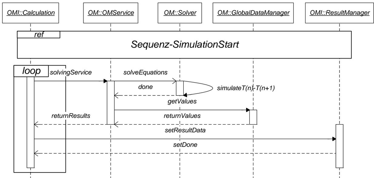
**Figure 6-6 UML-Seq Calculation phase**
