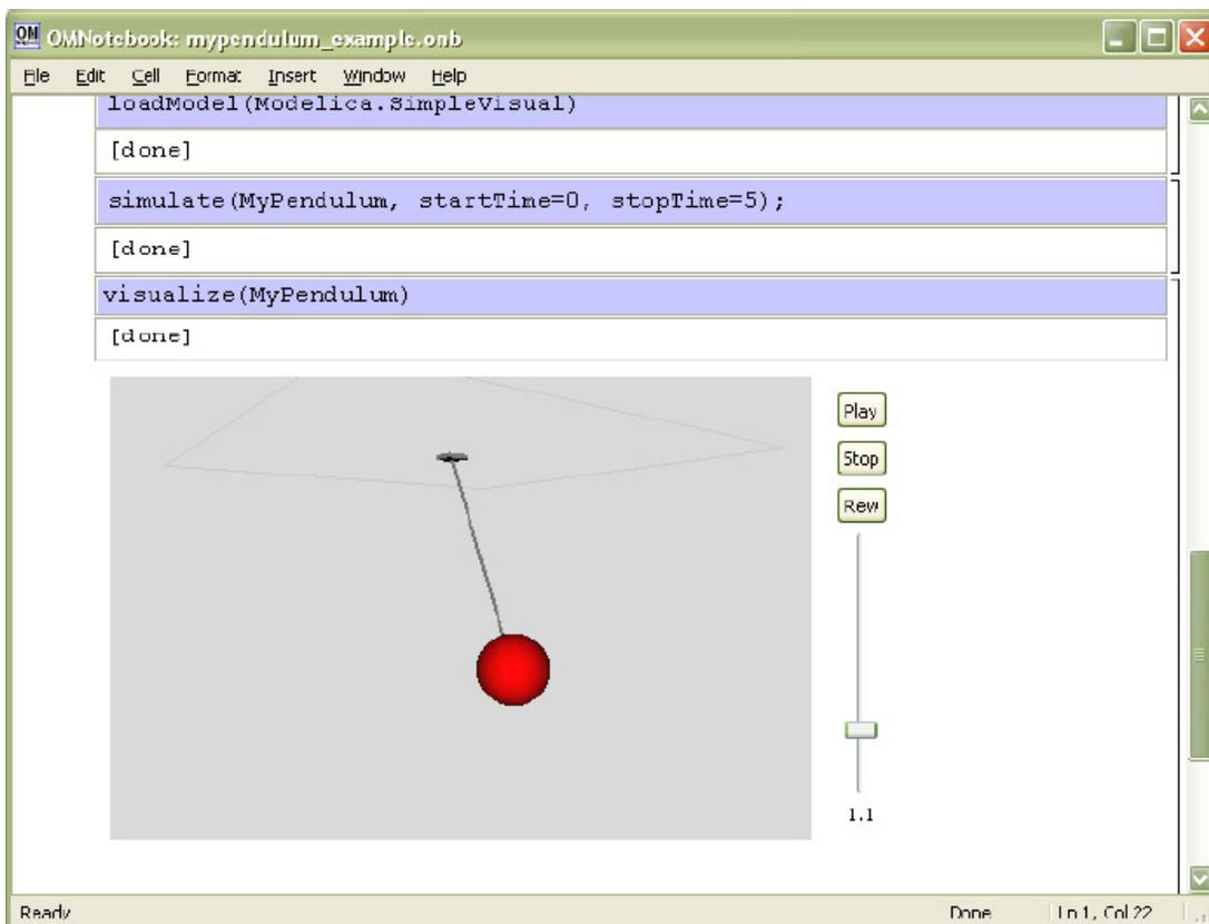
Figure 3-14. Visualization with animation of 3D pendulum.
