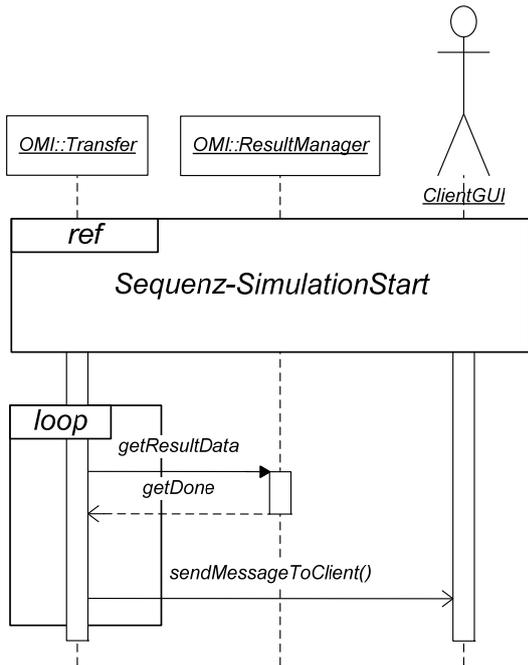
**Figure 6-7 UML-Seq Transfer to client phase**
