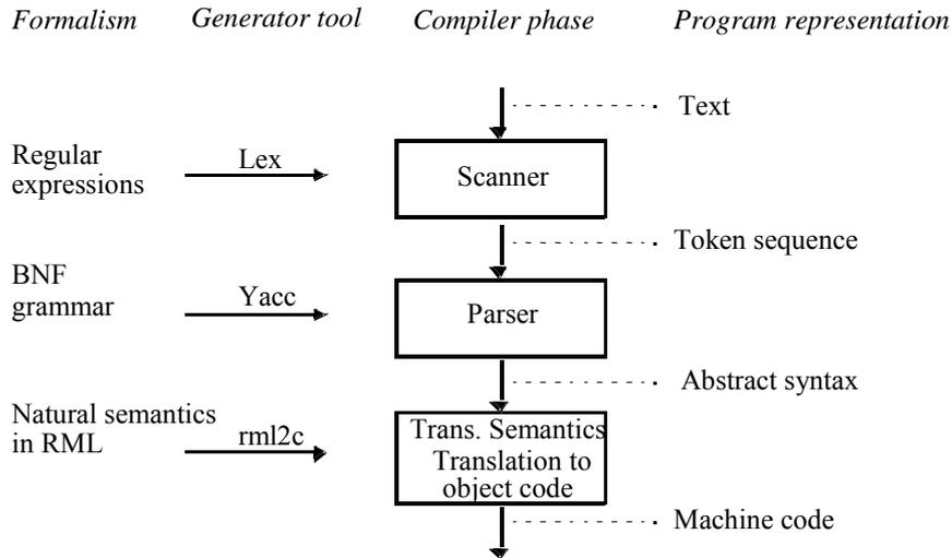
**Figure 3-2.** Simplified version of compiler generation based on translational semantics. The semantics of a language is specified directly in terms of object code primitives. In comparison to Figure 1-1, the optimization and final code generation phases have been excluded.
