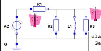
A more specialized class `TemperatureElectricalCircuit` is created by changing the types of `R1`, `R3`, to `TempResistor`
