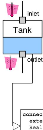
We would like to extend the Tank model to include temperature-dependent effects, analogous to how we extended a resistor to a temperature-dependent resistor
