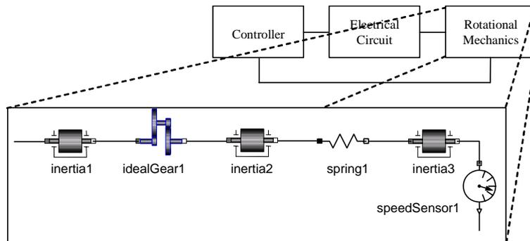
Modeling the mechanical subsystem including the speed sensor.
