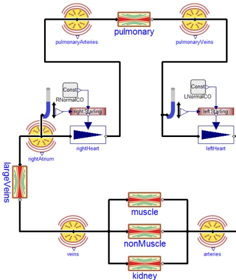
**Hydraulic:** resistor, pump, elastic vessel, hydrostatic column, inertia, absorption, ..
