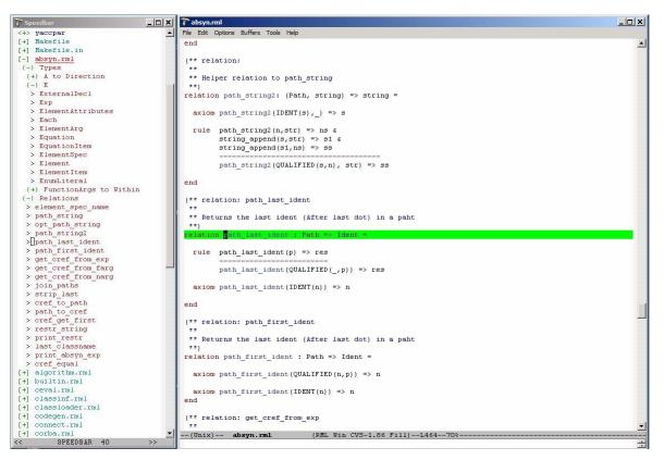
**Figure 4-1.** Emacs with a speedbar menu to the left, which allows clicking on file names (for expansion or closing the file contents menu). An expanded file shows all function, class, and type declarations. By clicking on one of those, you can position the editor at the appropriate definition.
