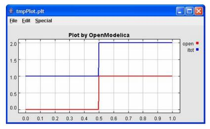
We note that the variable open switches from false (0) to true (1), causing itot to increase from 1.0 to 2.0.
