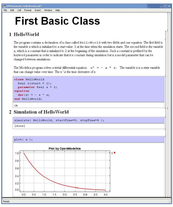
Figure 3-3. The HelloWorld class simulated and plotted using the OMNotebook version of DrModelica.
