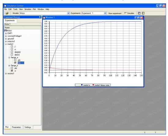
**Figure 2-8.** MathModelica plot window created after a simulation of the Motor model, using the full version of the MathModelica System Designer Graphic Editor (plotting not available in the MathModelica Lite version).
