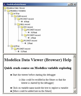
Figure 6-3. Modelica Data Viewer (Browser) for data structures, here a small abstract syntax tree.
