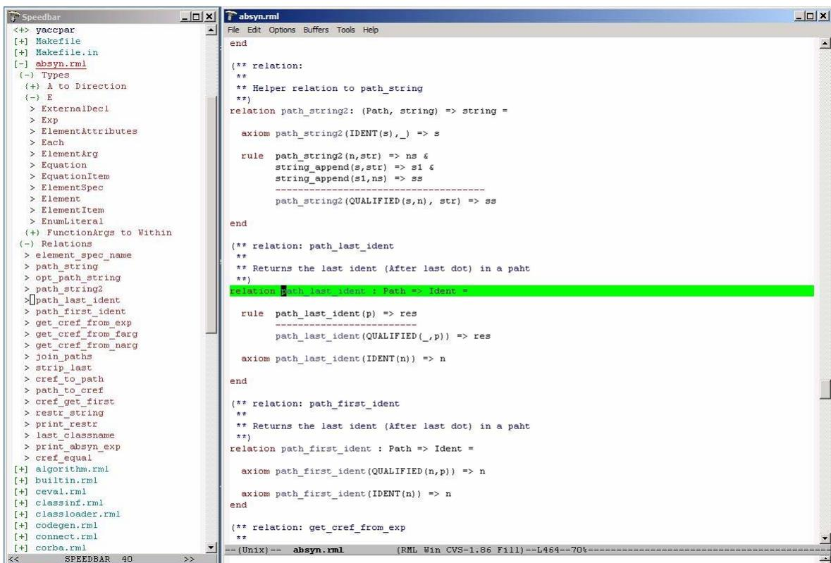
**Figure 4-1.** Emacs with a speedbar menu to the left, which allows clicking on file names (for expansion or closing the file contents menu). An expanded file shows all function, class, and type declarations. By clicking on one of those, you can position the editor at the appropriate definition.
