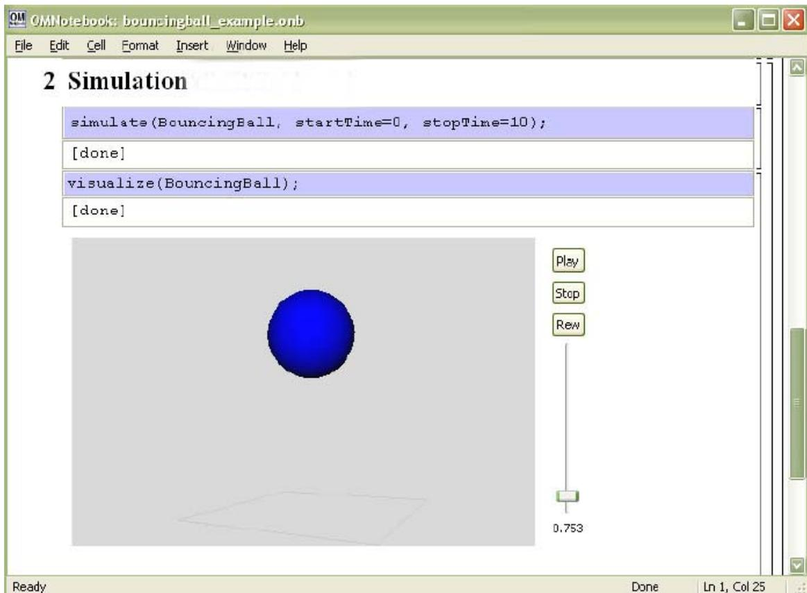
Figure 3-12. 3D animation of the bouncing ball model.
