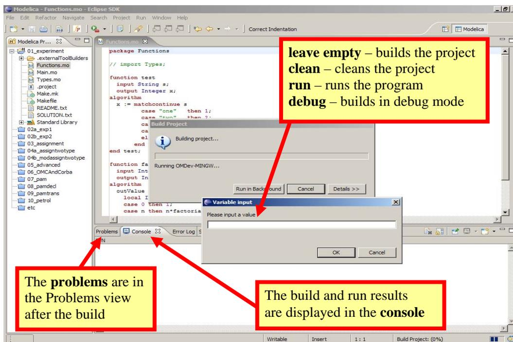
Figure 5-5. Eclipse – building and running a project.
